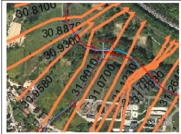
Fig. 5.4.2-1: Connection of a secondary branch to the main branch using snap mode during digitalization
